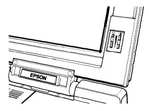
The contrast lever on the right determines how bright the characters appear against the background. To increase the contrast, move the lever up. To decrease it, move the lever down.
